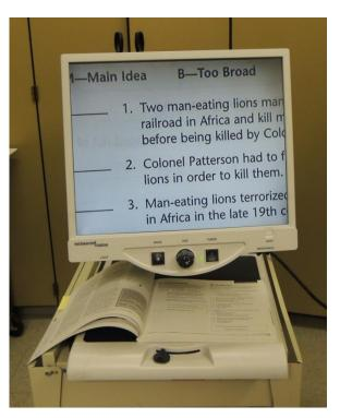
This is a CCTV. A CCTV is a system that uses a stand-mounted camera to project a magnified image onto a monitor.
