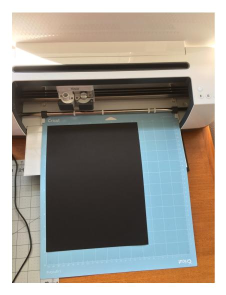
Now click on the weight cardstock you are using (Light Cardstock or Medium Cardstock) and press the blinking arrows on your Cricut machine, then the blinking "C" when prompted.
